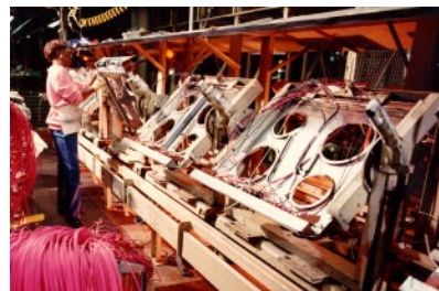
Parts advance through the wash process prior to painting.
