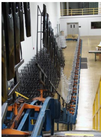
WideTrak conveyors easily negotiate horizontal and vertical curves.
