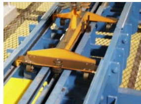
The three rail design stabilizes parts carriers.
