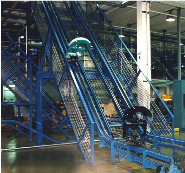
Motorcycle fenders are transported to storage after powder coating on an inverted Power & Free conveyor.
