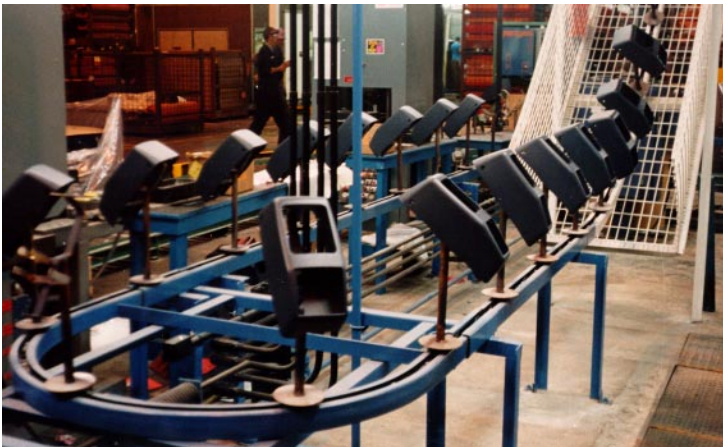
"C" hook attachments on an inverted power only track design helps to prevent product contamination.
