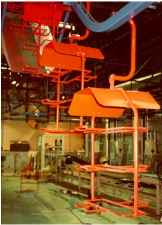
"C" hook attachments on an inverted power only track design helps to prevent product contamination.
