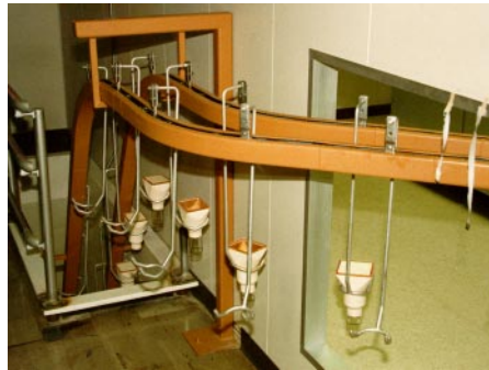
"C" hook attachments on an inverted power only track design helps to prevent product contamination.
